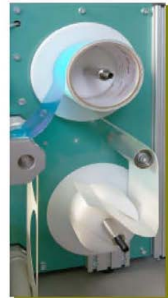
Clamp wax paper in the slot of the shaft / wax paper Stick up clamp top in front, twist slots against each other easily and fix clamp top
